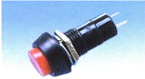
JX4855A SWITCH PUSH -BUTTON 125V a.c.3A CHANGE OVER PUSH-ON , PUSH-OFF 12 X 13 mm
